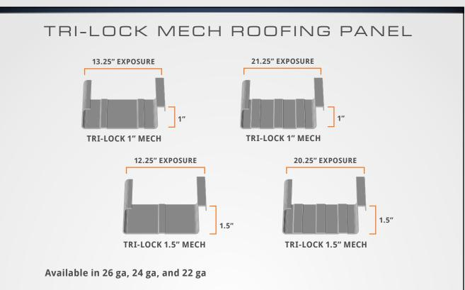
Profiles 1" Rib Height - Exposure Options - 13.25" 17.25" 21.25" Profiles 1.5" Rib Height - Exposure Options12.25" 16.25" 20.25"
